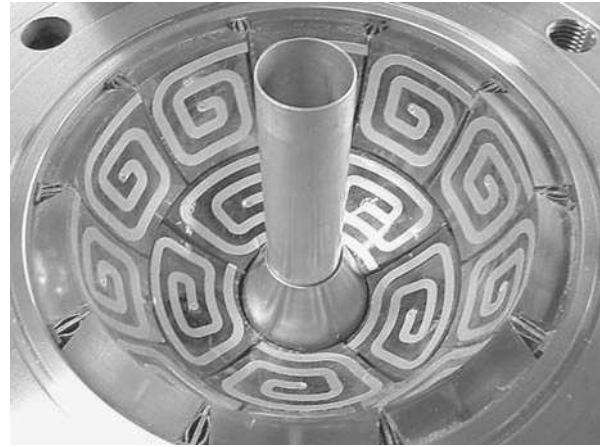
Fig. 3 Lithium tube in the center of a half tank
